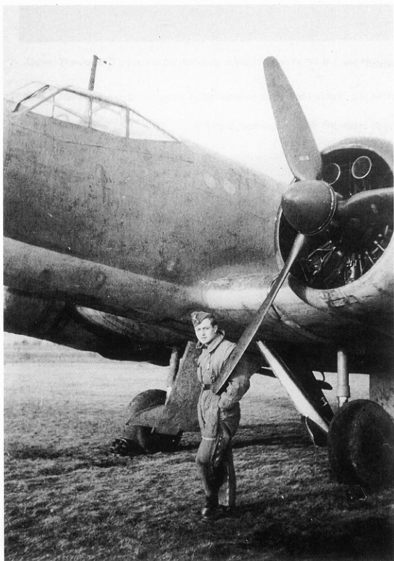
Left: Gefreiter Haferland stands in front of his machine. Notice the massive BMW 132 radial engine.
