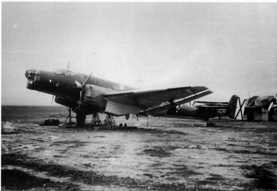
Below: This landing gear damage is being repaired at the Leon airfield. The aircraft in the background is an He 70 from the Condor Legion.
