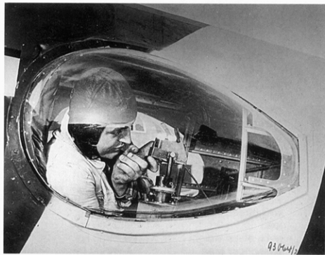
At least one Ju 86 D was used for testing remote-controlled guns, necessary for arming high-altitude combat aircraft and bombers. The two sighting cupolas bear a strong resemblance to those used on the Ju 288 prototypes.
