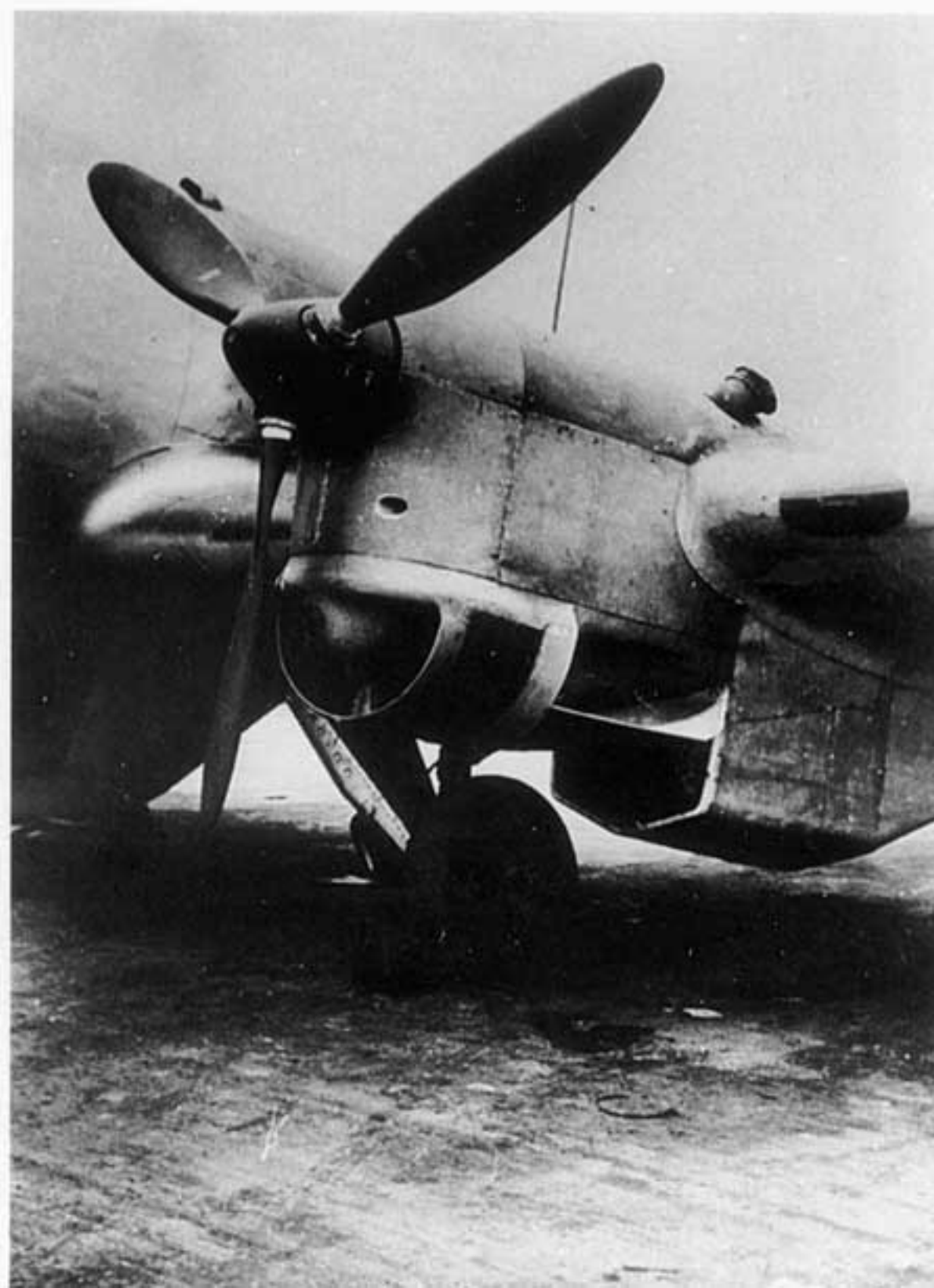
Right: An exceptionally large radiator airscoop was necessary for the Jumo 207 to operate at high altitudes.
